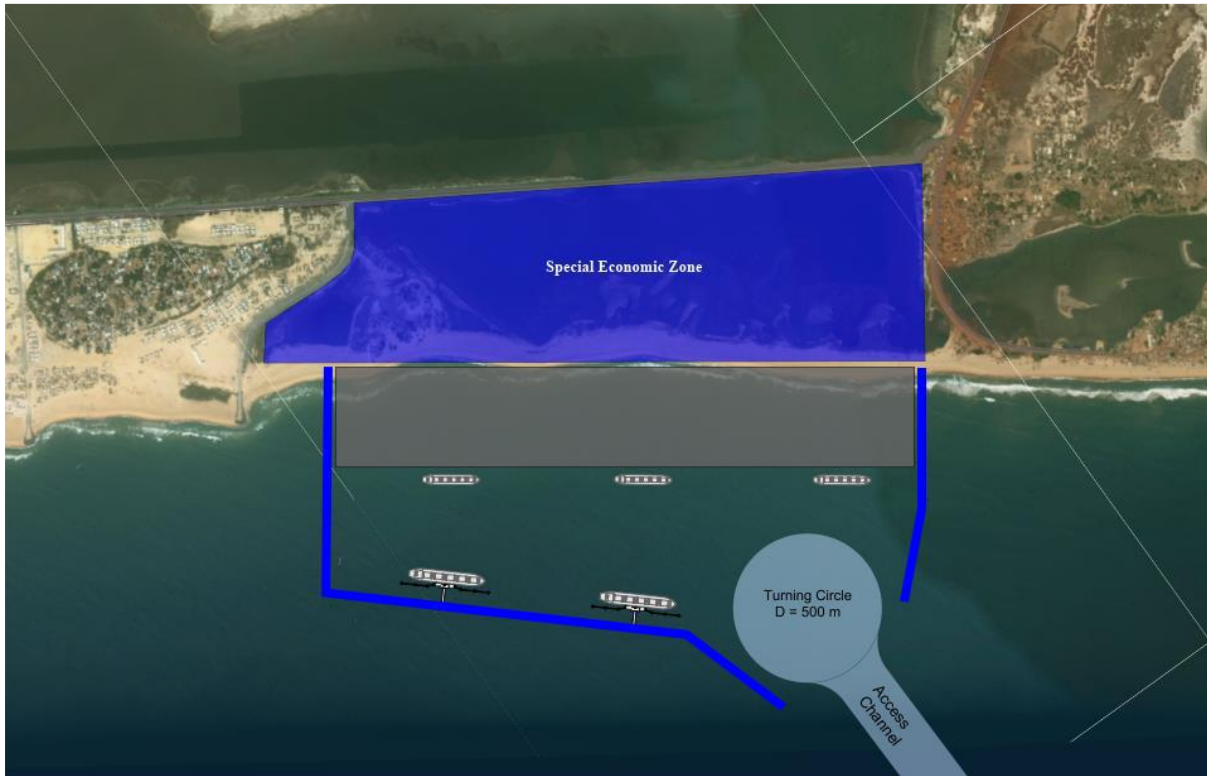
Figure 5-1 - I-Shaped Port Configuration (Source: SIIPS, 2021)
