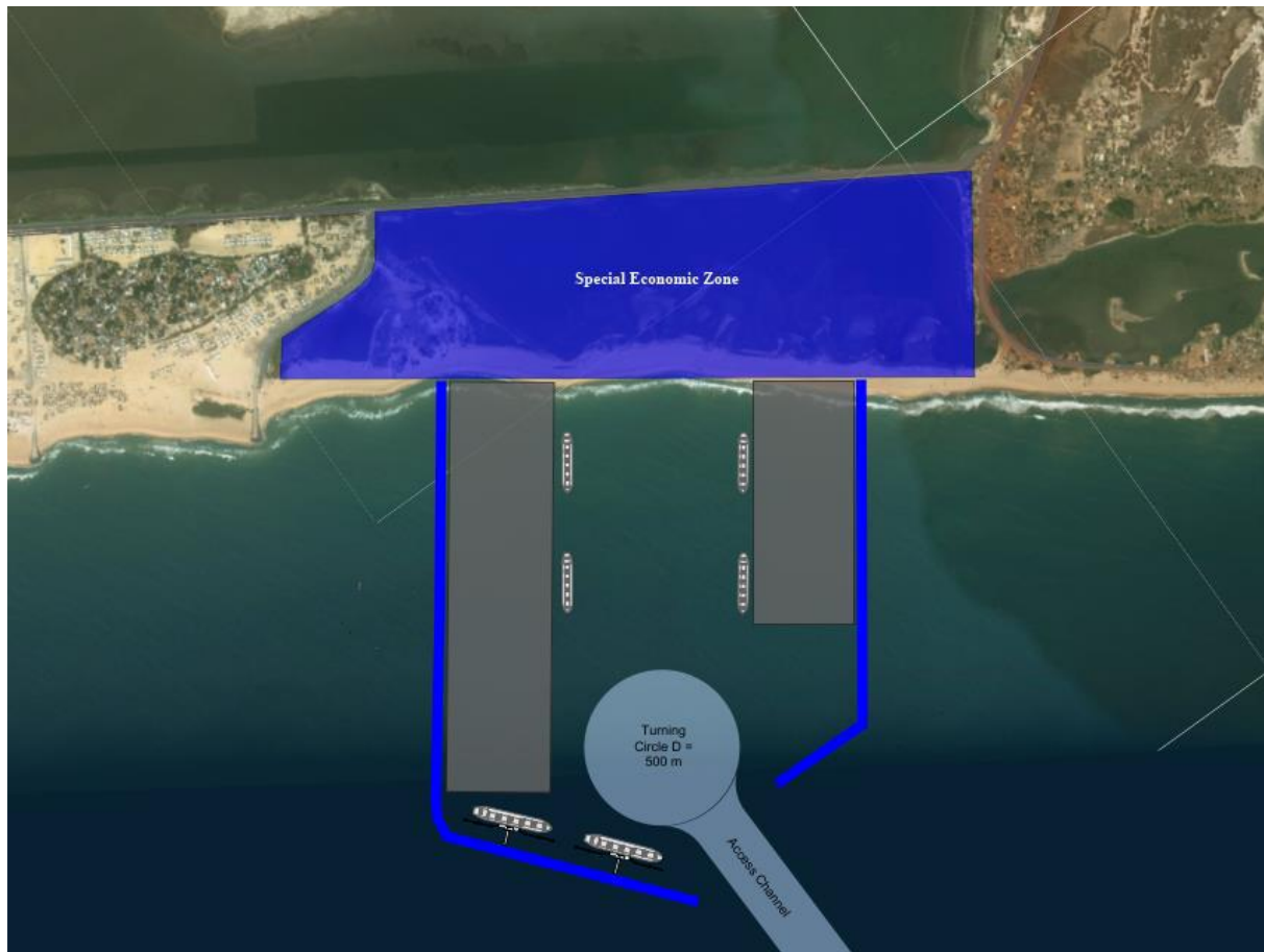
Figure 5-2 - U-Shaped Port Configuration (Source: SIIPS, 2021)
