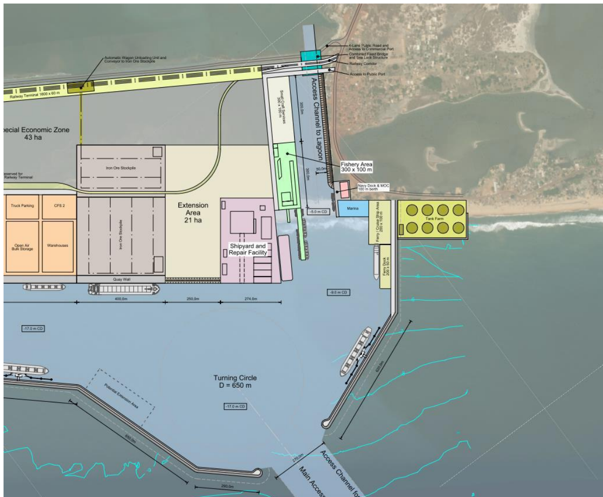
Figure 5-4 - Potential Alternative Hydrocarbon Terminal Location (Source: SIIPS, 2021)
