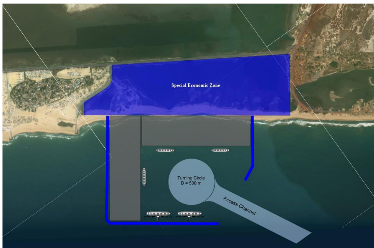
Figure 5-3 - L-Shaped Port Configuration (Source: SIIPS, 2021)
